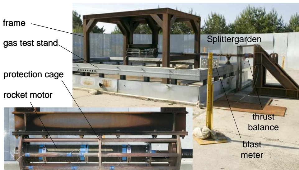
Figure 5: Fast Heating gas-fire test stand with motor thrust-balance set-up.
