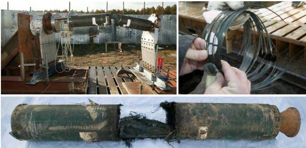
Figure 3: Bullet Attack test, case damage.
