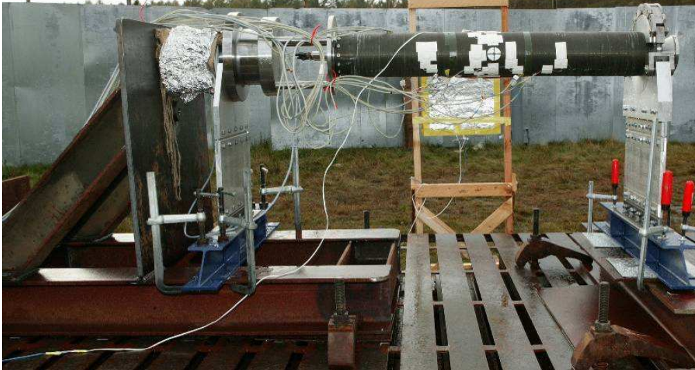
Figure 2: Bullet Attack test set-up, IM-motor on thrust-measurement test stand.
